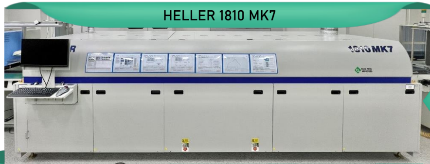
10 Zone Reflow Oven with Static Pressure Computer Fan Speed Control of Heater Module Blowers
