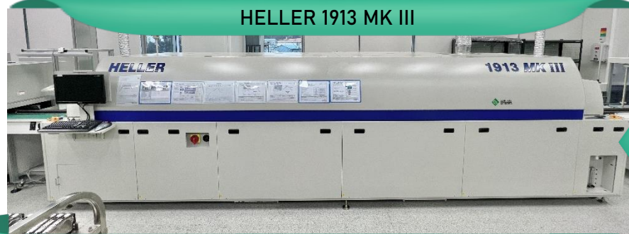
15 Zone Reflow Oven with Static Pressure Computer Fan Speed Control of Heater Module Blowers
