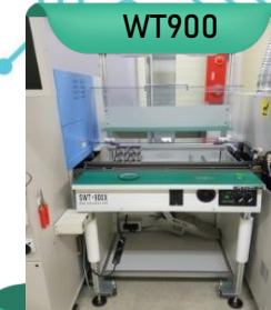
VISUAL INSPECTION (mounting status)
